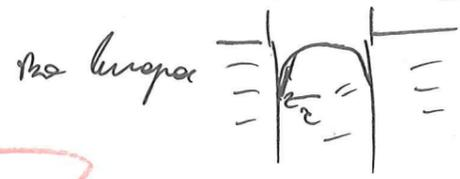
$\rho g h_1 = 2 \cdot \frac{4\sigma}{\gamma} \Rightarrow 2 \rho g h_1 = 2 \frac{\sigma}{\gamma} = \rho g h$
