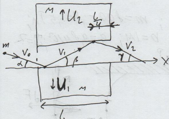
$$V_1 = V_0 \frac{\cos \alpha}{\cos \beta}; V_2 = V_1 \frac{\cos \beta}{\cos \gamma} = V_0 \frac{\cos \alpha}{\cos \gamma}$$
